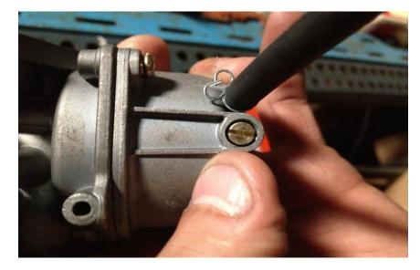
(to drain the bowl, loosen this screw until all the gas has dumped out, use a bowl to catch the gas. You will see a yellow/brown/orange liquid come out with the gas, this is just packing liquid for shipping. Once this has all drained out, screw back tight, put the capped fuel filter back on the fuel line and fill the tank with gas)
